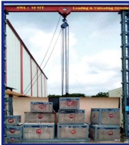
Available Dead Weight Blocks Upto 38.25MT (Various Capacity)
