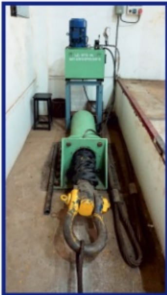
Horizontal Hydraulic Test Bench SWL : 150 MT, Length : 18 Mtr
