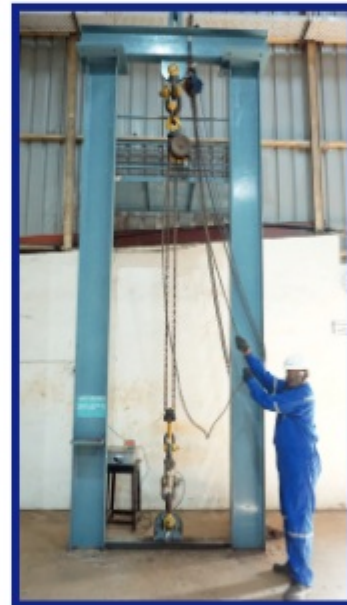
Vertical Test Bench SWL : 30 MT, Height : 5.2 mtr
